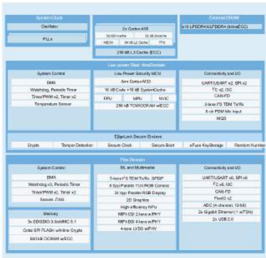
Figure 2: i.MX 93 SoC Block Diagram
